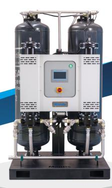
Mentis S-PSA50 Oxygen Generators Produce  $55Nm^3$  of gaseous oxygen per hour at  $93\% \pm 3\%$  oxygen concentration at up to 6.0 bar oxygen outlet gas pressure.
